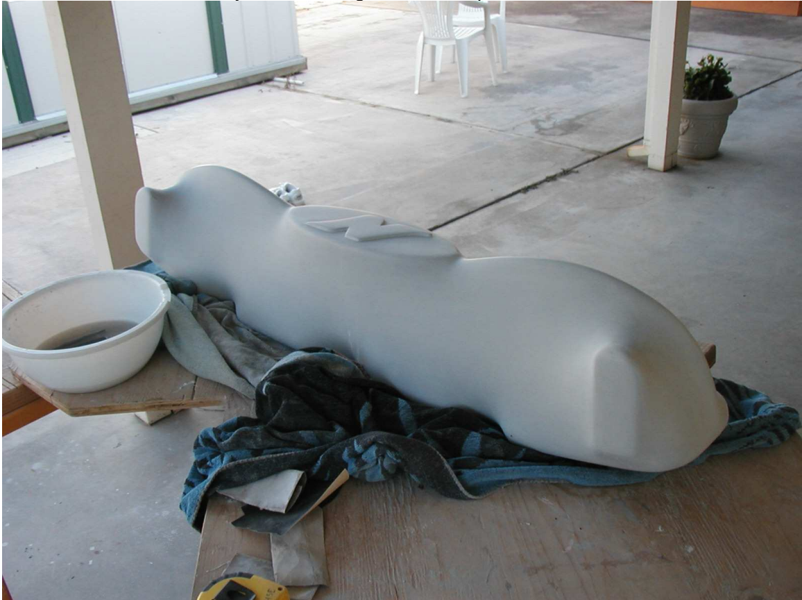
Smooth sanded and ready for mounting holes and speaker wire holes.
