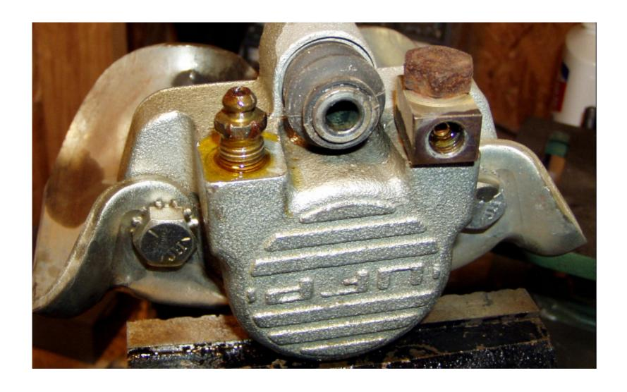
Once the screw is out, evaluate the condition of the caliper. This one has a lot of rust in it. The caliper is a UFP DB-42 on the tandem Ameratrail trailer. They are available here. There are different part numbers for left and right.
