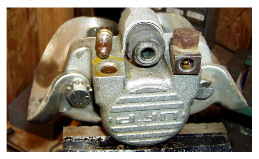
Reattach caliper, replace brake pads if necessary. Mine were fine. They are plymouth acclaim brake pads according to the trailer documentation. Hook up the brake lines. Attach a length of clear tubing to the bleed screw on the (boat) driver side rear. Run this tube into a clear container, fill it partially with brake fluid and submerge the end of the hose. Loosen the bleed screw.
