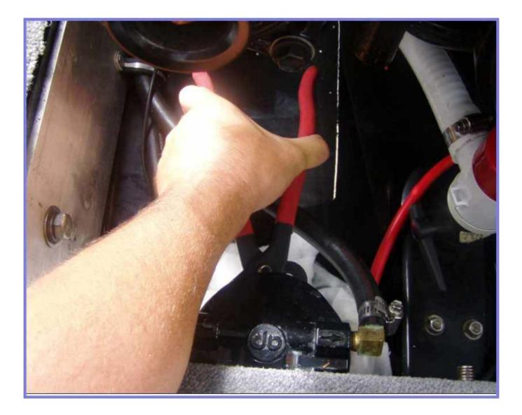
Check the removed filter to see if the O-ring gasket came off with it. Spin the new filter on by hand, tighten as much as possible by hand. Make sure that you do not install a filter on top of an old O-ring. Clean up all spilled gas and let the engine compartment air out.
