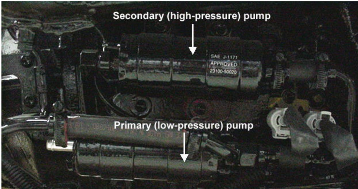
Fuel Pump No.1, which is the second pump in the fuel line, is listed as part number 2310150020 is the secondary, high-pressure fuel pump on all models of Epic boats.
