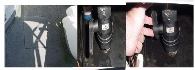
Fill Instructions: Operate at slow speeds. Open valve located under floor battery hatch. Valve handle in up position is open.
