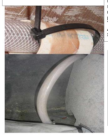
Running hose to port fill are via bilge or starboard walk thru area. Up along wire run to top of trunk bulkhead. Direct to port phat sack bag fitting. THE FILL HOSE MUST RUN AS HIGH AS POSSIBLE TO PREVENT SYPHONE FILLING OR DRAINING.
