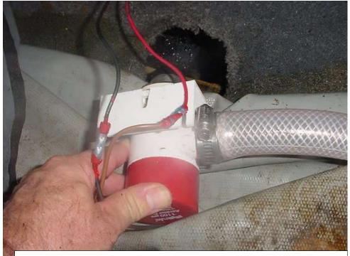
Located in trunk Install new Drain pump located under center bottom of ballast bag. Remove check valve.
