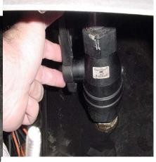
Fill Instructions: Operate at slow speeds. Open valve located under floor battery hatch. Valve handle in up position is open.
