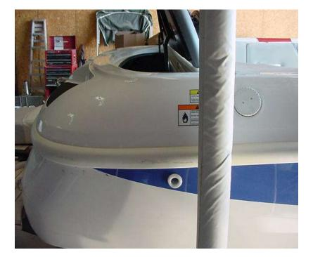
Drill hole Aft of vent hose.
