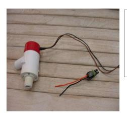
Cut out old connector and use heat shrink butt connectors on wire.
