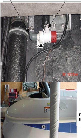
Drill 1 1/8 hole towards stern of vent thru- hull
