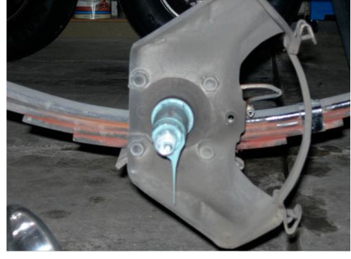
Find a small seal driver that will pass through the hub and seat into the inner bearing.
