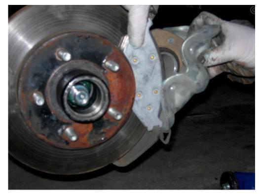
Insert the retaining wire.
