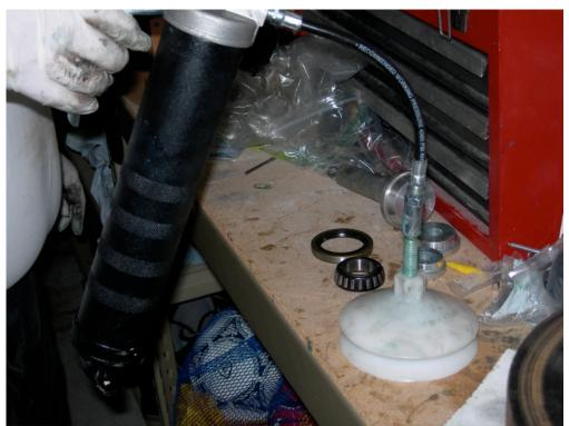
Remove the bearing from the packing kit.
