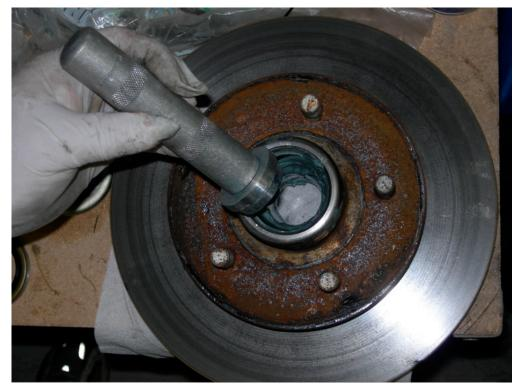
Knock out the inner bearing and inner seal.
