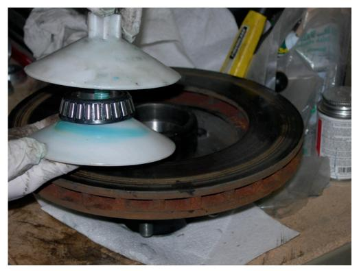
Pack the bearing using marine grade wheel grease.
