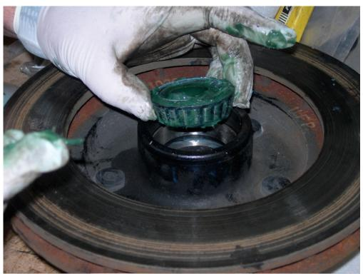
Tap the inner seal into the hub using wood block.
