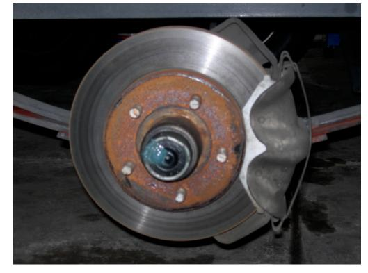
Remove the retaining wire.
