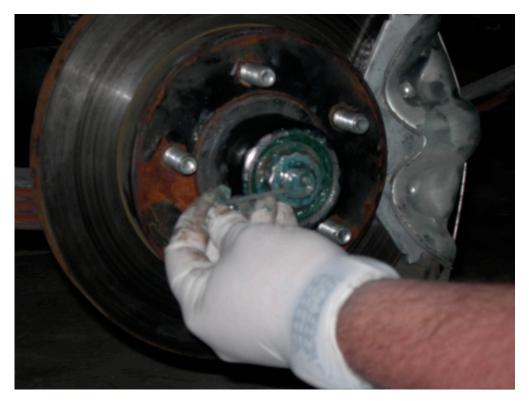
Pump marine wheel grease unto the hub until you see grease oozing out around the washer.
