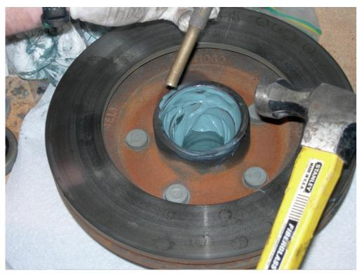
Note - you'll need to ease the outer race/cup out by tapping the race around different points to inch it out.
