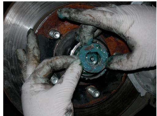
Insert the bolt and thumb tighten while rotating the hub/rotor. When the hub/rotor binds slightly, back off the bolt/nut I/6 to I/4 turn. The hub/rotor should spin without any resistance.
