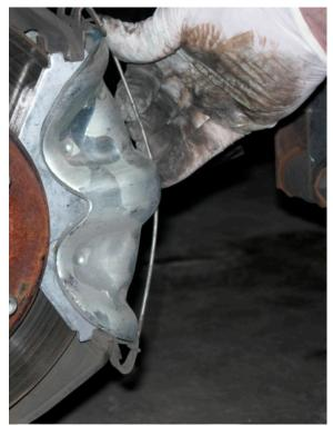
Remove the Caliper and brake pads.
