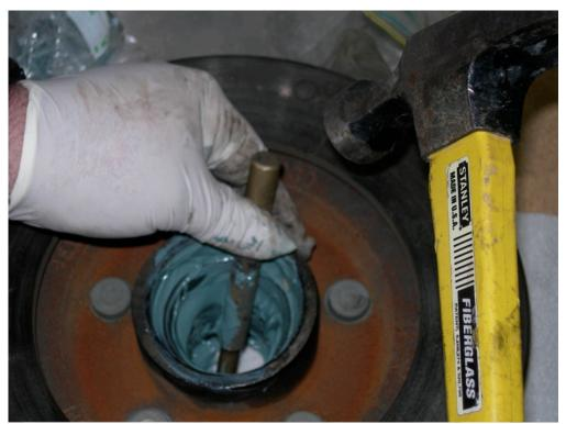
Discard the old outer race. Remove the inner race the same way by tapping it our using the brass drift punch.
