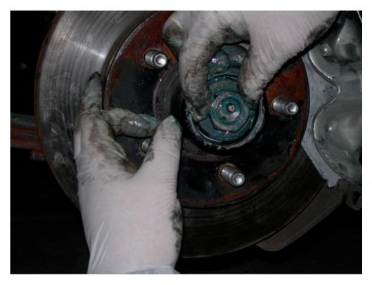
Place the safety nut onto the hub nut.
