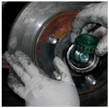
Pull the wheel hub/rotor off the axle spindle.
