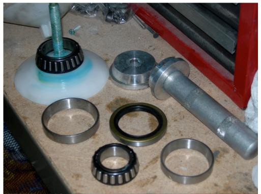
Insert the new outer race/sup using the drive tool with the appropriate sized driver. Make sure the race/cup is seated straight and all the way into the hub.
