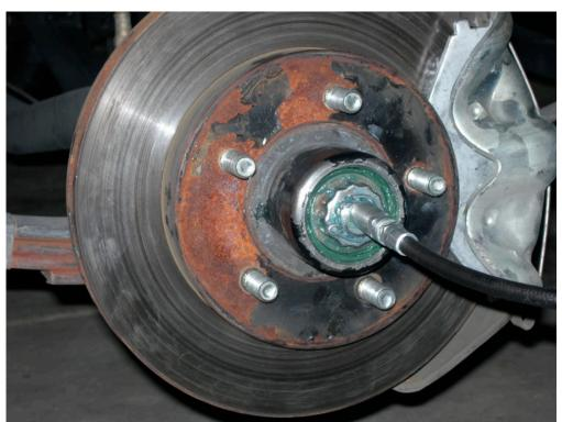
Tap the hub cap or buddy bearing onto the hub.
