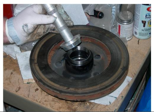
Place the inner bearing into the bearing packing kit.
