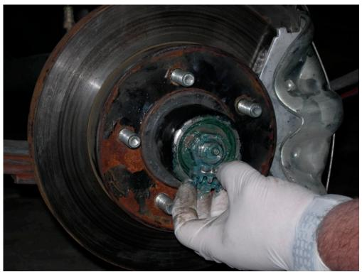
Insert the cotter pin. Bend and wrap both ends of the cotter pin.
