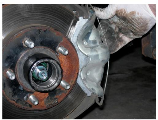
Insert the outer bearing.
