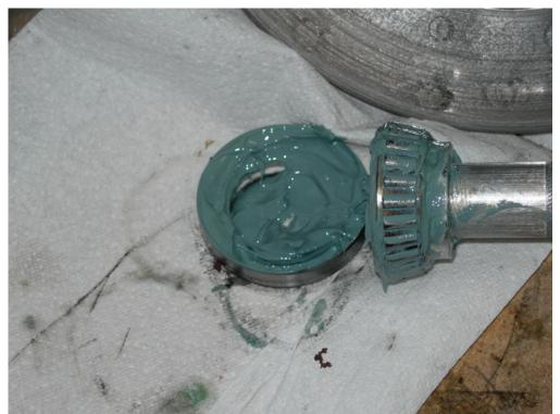
Knock out the outer race/cup using the brass drift punch.
