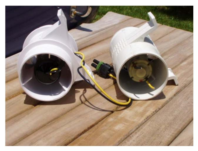
To remount blower, insert a drill bit in the forward mounting hole. slide the blower mounting hole over the bit. Make sure the blower flow is going UP. Put the aft screw in first, then remove the bit and start the forward screw.
