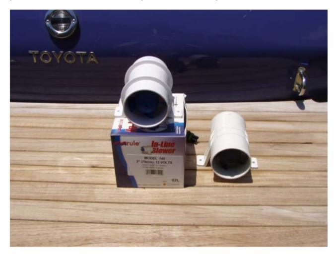
I cut the connectorized wires off the original blower and soldered and heat shrank the leads to the new blower. I hid the splice inside the blower.
