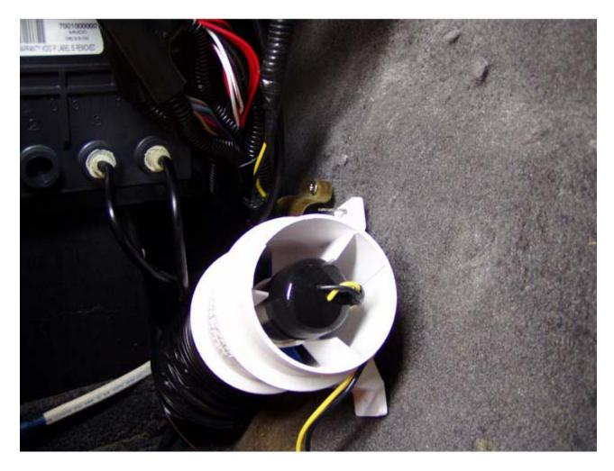
Connect the connector and secure the hose with the new ties provided with the blower. If you are missing any hull plugs, get them from the dealer. Test the blower, you should feel air coming out of the black transom plates on the stern.
