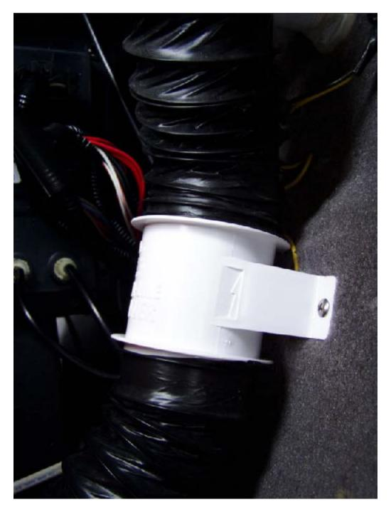
The original Attwood is LOUD and inefficient. To remove, cut the wireties top and bottom, separate the connector (yellow and black) Remove the two sheet metal screws from the hull plateholding the blower. The new blower footprint is identical.
