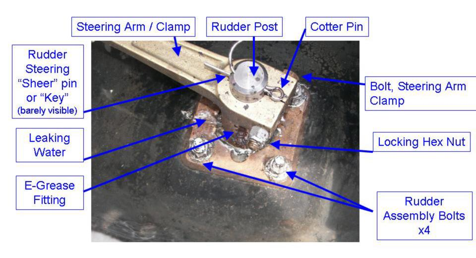
To access the rudder assembly there is a removable plate in the stern gear locker... (At least this is where it is on S22)
